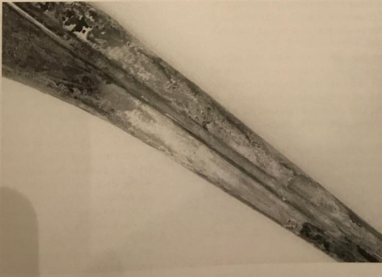
FIG. 4. Intergranular corrosion is demonstrated on this etched stainless steel specimen.
