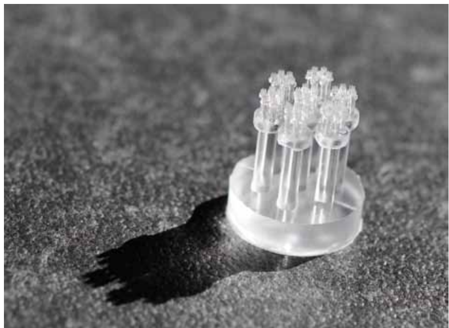
Figure 2: Macroscopic hierarchical model system with three levels of hierarchy.
