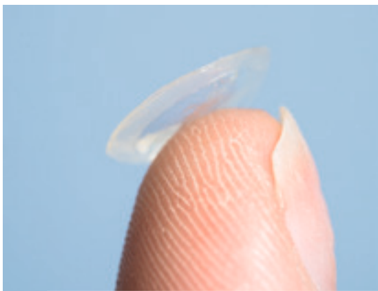
► Fig. 1: Laboratory prototype of a self-lubricating contact lens containing biofactories of hyaluronic acid.
