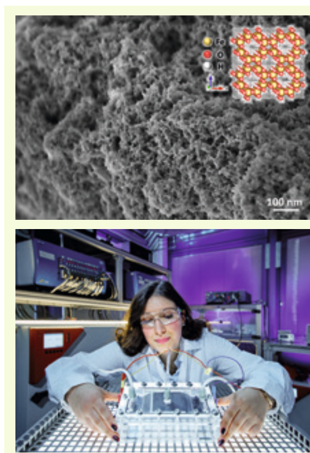
► Fig. 1: Microstructure and crystal structure of iron hydroxide. Fig. 2: Cell for electrochemical lead removal.
