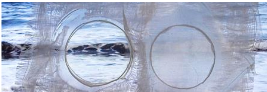
Glass fiber reinforced polymers, left, correct, right, incorrect matrix
