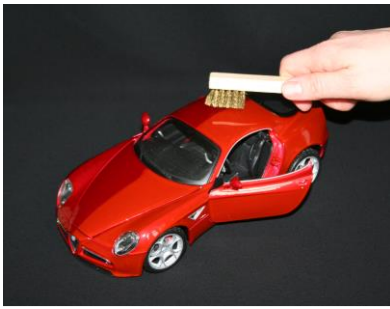
Superficial micro-scratches on top-coat
