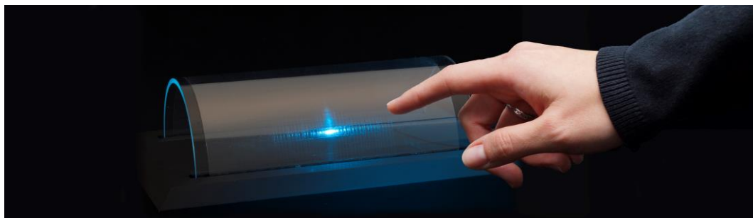
Flexible touchscreen – by inkjet printing of new TCO inks on PET foil
