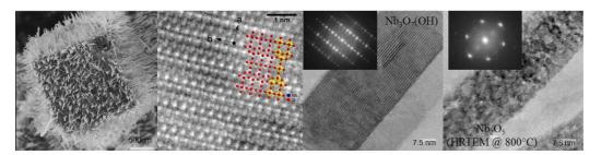
Scanning electron microscopy image of a novel 3D nanoarray (left) [1]; high resolution TEM image showing the atomic structure (middle) [1]; and in-situ high resolution TEM images (right) acquired at room temperature and at 800°C revealing the thermally induced phase transformation [3].
