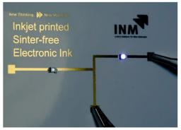
Printed circuit with electrically conductive ink from INM ©INM; freely used in connection with this news story. The illustration can also be found <u>here</u>.
