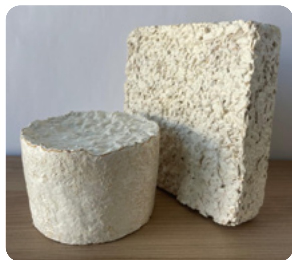
Fig. 2: Mycelium-based composite from the LoopOfFun project. Organic waste was bound to a composite by mycelium-based fibers acting as binder.
