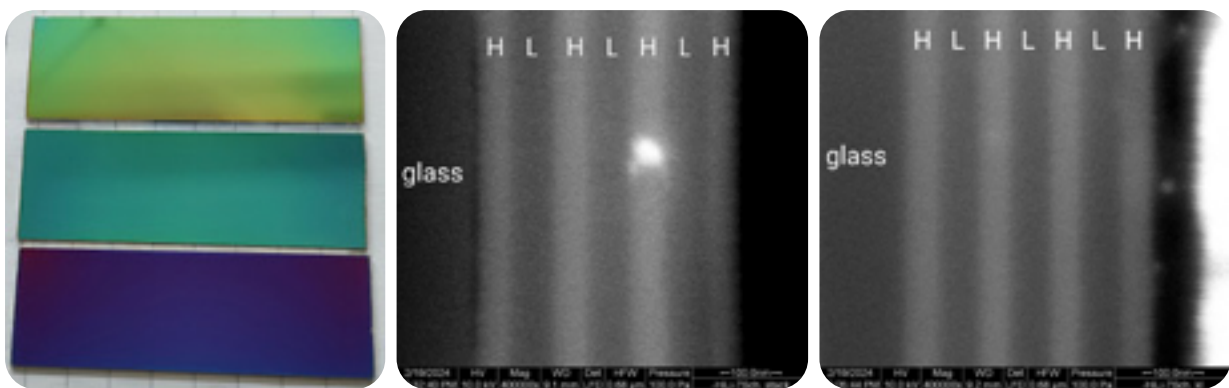
► Fig. 1: Live Mirror: Silver mirrors coated with several layers of different thicknesses of aluminum and aluminium oxide
