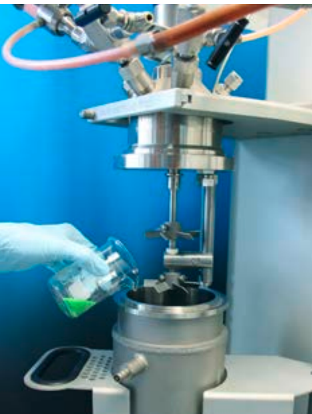
► Fig. 1: TEM image of BaTiO 3 nanoparticles in cured polymer matrix // Fig. 2: BaTiO 3 nanoparticle synthesis in an autoclave
