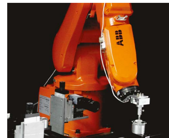
▶ Fig. 1: INM's Gecobot demonstrating switchability of the adhesion strength for utilization in pick and place operations has drawn much industrial interest: switching by fiber re-orientation. Fig. 2: Commercial 6-axis robot equipped with lab-produced Gecomer technology.
