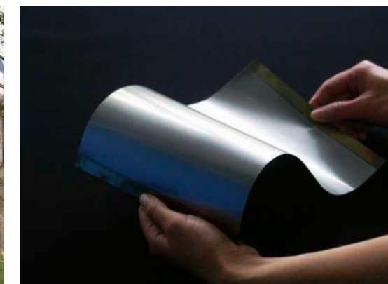
▶ Stainless steel foil coated with a glass like system for flexible CIGS solar cells.
