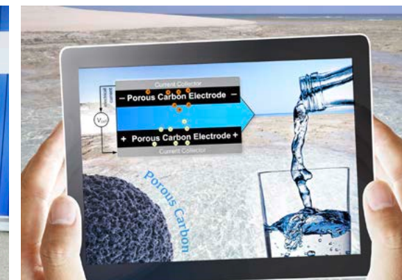
► Concept of capacitive deionization.
