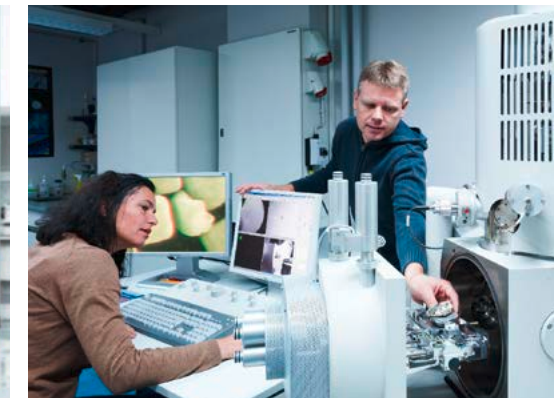
▶ Loading of a sample in the environmental scanning electron microscope for a service project.
