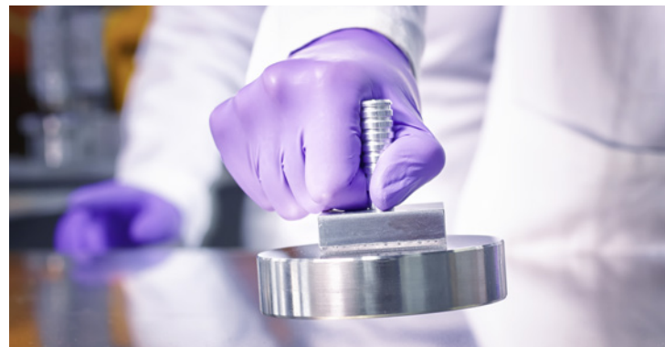
► Fig. 1: Bioinspired micropatterned adhesive as platform of patented Gecomer Technology. Fig. 2: Demonstration of adhesion performance.
