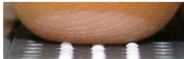
► Fig. 1: Neural processes evoked by changes in friction between the fingertip and a Braille display were investigated by means of an electroencephalogram (EEG). Fig. 2: Programmable Braille display in interaction with the finger of a participant. The friction signal depends on the strength of contact and on the number of Braille dots raised.
