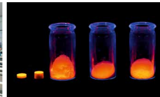
▶ Luminescent samples of scintillator nanoparticles.
