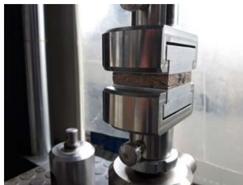
► Fig. 1: Determination of mechanical properties: NaMiComp fibreboard specimen in bending and transverse tensile test.
