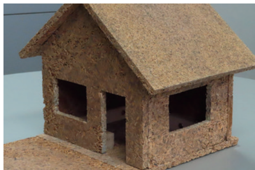
► Fig. 1: Self-healing behavior of polyrotaxane containing coatings as top-coat on painted surfaces at 90 °C. Fig. 2: Fire-proof acacia-fiberboard demonstrator house fabricated exclusively from Namibian precursors.
