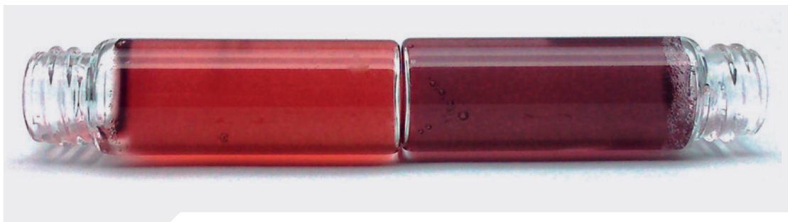
► Fig.: This active nanocomposite reversibly changes its color upon stimulus (in this case, when a certain temperature is reached). It contains mobile “plasmonic” metal nanoparticles that rearrange and change the color.
