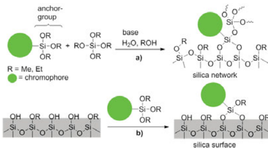
Figure 1. Covalent dye doping a) in situ dye incorporation, b) dye functionalization after particle synthesis
