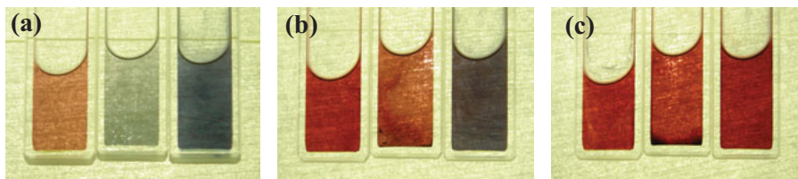
Figure 1. AuNPs of 3.7 nm radius covered with C16 thiol in hexane (left), decane (middle) and hexadecane (right) at (a) 20°C (b) 35°C and (c) 55°C.
