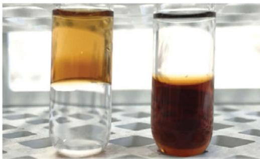
Figure 1. Phase transfer of magnetite nanoparticles from n -hexane to water in presence of modified PMA.
