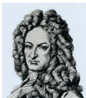
► On the occasion of the 300th anniversary of Leibniz' death in 2016, we discovered a rather small Leibniz by scanning electron microscopy. The wig of this nano-scale sculpture was formed by the transfer of gold to the tip of an atomic force microscope in repeated cycles of a friction experiment.
