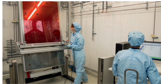
▶ Wet coating equipment for very thin layer developed at the InnovationCenter INM .
