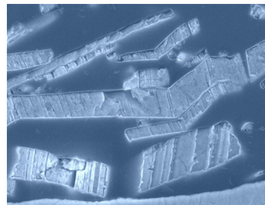
► Cross section of a corrosion protection layer containing zinc-phosphate flakes (magnification 12500 x).
