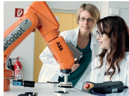
► INM's Gecobot for demonstration of novel pick & place processes using bioinspired adhesion devices.
